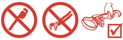
Proper care must be taken when threading a plastic valve into a piping system or failure of the valve body may result:
